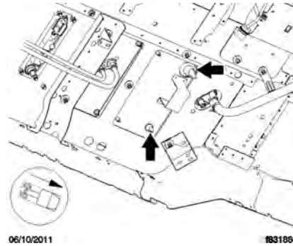
Fig 117, Drain Tube Inspection
